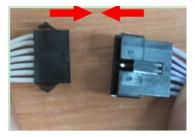
FIG-17 Connecting control panel connectors
