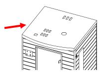
FIG 19 Slip the power cord through Roof Cover
