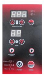
Power On/Off: Press to control the main power of the sauna
