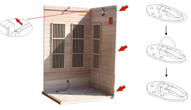
FIG 5 Assembling Right Side Panel
