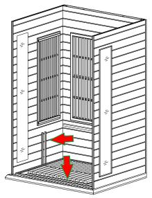
FIG 8 Placing Floor Heater
