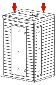
FIG 12 Installing Roof Cover
